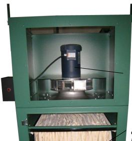
3 HP TEFC motor with direct drive forward curved blower
